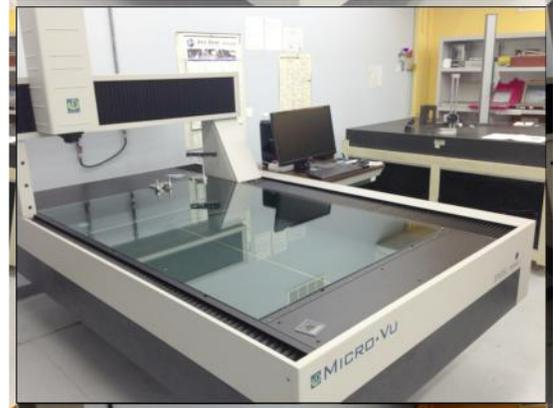
**CNC– Vision & Touch Probe CMM, (MICRO-VU 1604 UC, 41” X 65” X 15.7”)
